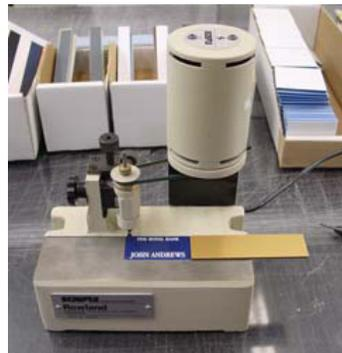
*It is faster to bevel short sides of plates together using a piece of scrap to "push" the material.*
