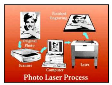
What makes this conversion from photo to engraving possible is the halftone screen. As in printing, the halftone screen converts the continuous tone gray values of the photograph to a series of large to small solid black dots that simulate the gray tones of the photograph. There are variations on the traditional halftone screen that will also work for photo laser engraving, but to avoid confusion, only the traditional screen method will be discussed.
