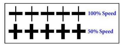
For high quality rendering, the recommended speed should be dropped to 50%, and the power setting needs to be adjusted to a corresponding percentage that will allow the cap to be burned through. Higher power settings than needed will
