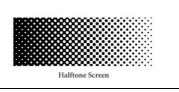
When we look at a magazine photograph, we are convinced we see different shades of gray when actually we are looking at solid black ink only. This black ink is printed in the form of tiny dots in patterns that are usually invisible unless magnified. In a traditional halftone screen, the dots are evenly spaced. Because they vary in size, you experience the illusion of looking at shades of gray.
